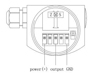
**Note:** Terminal "GND" should connect with shield wire of the cable, and the shield wire should be grounding reliably; or connect "GND" with housing terminal.
